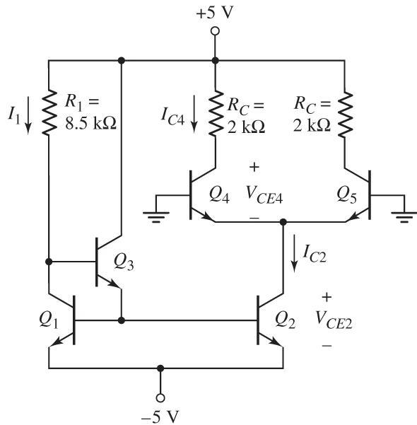
$$(ii) \quad I_1 \approx I_{C2} = \frac{V^+ - V_{BE3} - V_{BE1} - V^-}{R_1} \quad [2]$$
