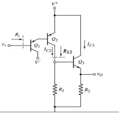
$$R_{i} = r_{\pi 1} + (1 + \beta) r_{\pi 2}$$
