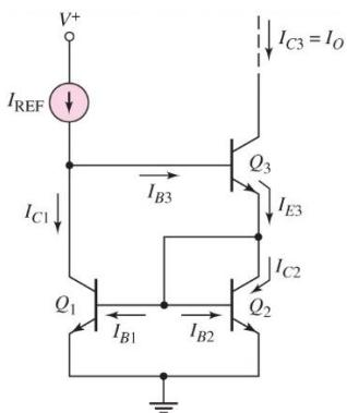
Placements of  $Q_1$ ,  $Q_2$  and  $Q_3$  [2 marks]Batteries  $V^+$  and  $V^-$  labels [2 marks]Currents  $I_{REF}$  and  $I_O$  labels [2 marks](ii) Both three-transistor and Wilson current sources have an increased stability [1.5 marks] with smaller  $I_O$  change [1.5 marks].
