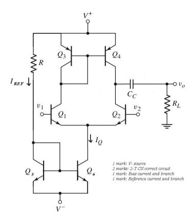
$$v_0 = g_m v_d(r_{02}||r_{04})$$
