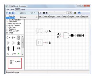
2. Note that the Oscope dialog box appears. To add inputs for the Oscope to plot, simply select them from the drop down box and they will be added to the plot. Note that when an input is added, another input box appears allowing you to add more inputs to the Oscope. Only TO gates in a circuit can be plotted.
