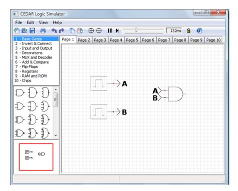
10. Drag the LED onto the canvas and connect it with the output of AND gates. Then, drag the "To Named Link" and connect it with the LED.
