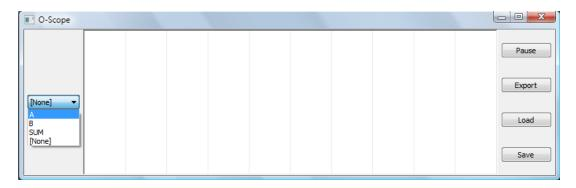
3. Add A, B, and sum to the Oscope plot so it looks as shown. Since the A input clock is twice as fast as the B input, the circuit's response to all possible inputs (0,1,2,3) can be observed.
