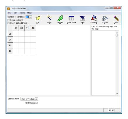
2. Fill the box with the value based on the standard SOP expression. Double click at the box to get the value "1". To get "0" on the box, double click the box twice.
